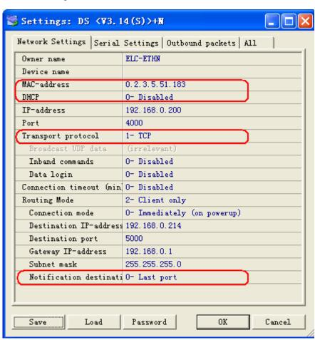
Note: Just as above figure shows, parameters in "Destination IP-address, Gateway IP-address and Subnet mask" must be adjusted to be exactly same as those in your PC. However, "IP-address" and "Port" in above configure shows can be adjusted as you like.
